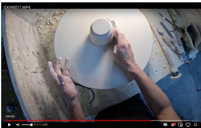
2'10" - 2'21" Smoothing the surface of the piece with sandpaper.
