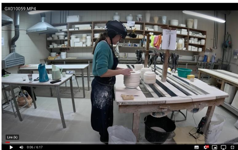
0'25'' - 0'30'' Using the cutter, she removes the demoulding ribs (« rainures de démoulage ») inside the pouring hole of the mould. During this operation, she rotates the mould (clockwise) with her left hand.
