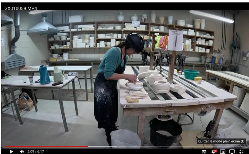
To cut the junction points of the handles, she leans her body towards the mould and uses fairly airy movements, lifting her hand and wrist so as to touch the piece as little as possible, without exerting pressure on it so as not to deform it.
