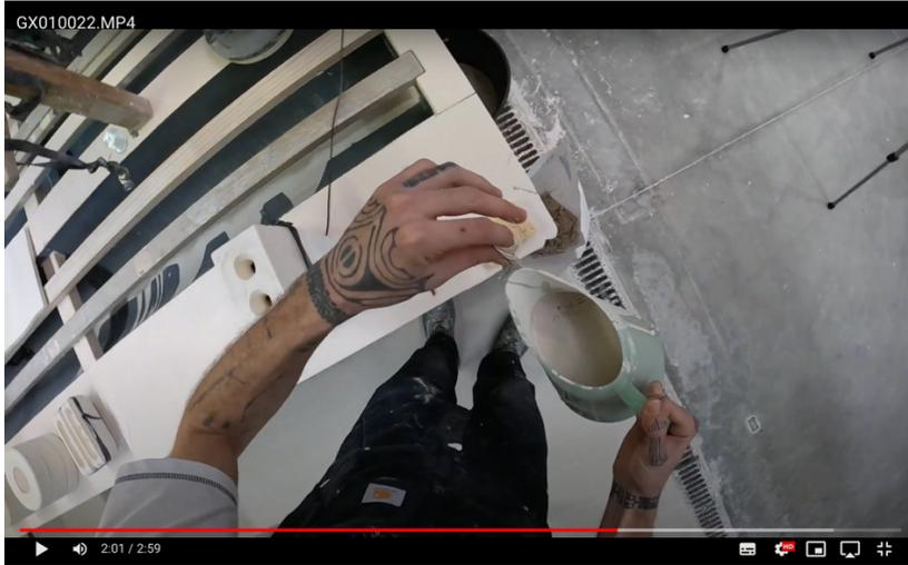
2'03'' - 2'15'' He fills the mould by pouring slip liquid into just one of the pouring holes.
