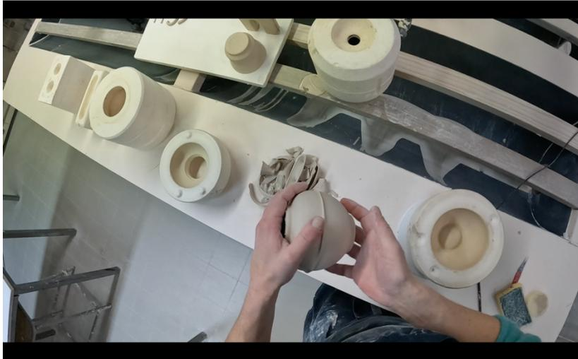
5'42" - 6'11" She repeats the operation with the last mould: she opens it with the blade of the cutter (using rapid movements of the right wrist), taps to detach, and demoulds another piece with rounded shapes.
