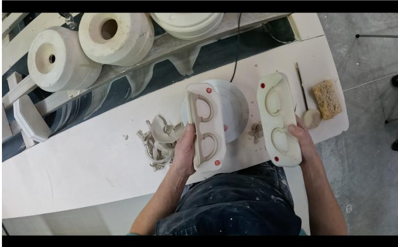
5.5. TRIMMING AWAY THE EXCESS SLIP FROM OF THE INTERIOR OF THE MOULD (with a sharp scalpel)
