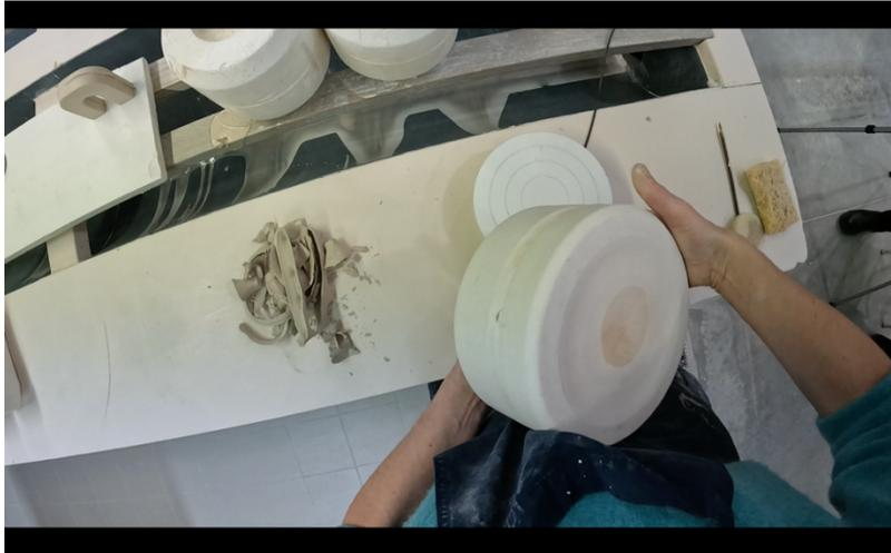
Turning the mould to demould the piece
