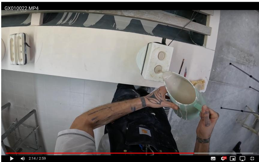
2'24'' - 2'38'' He pours slip into two moulds that are held together with a rubber band.
