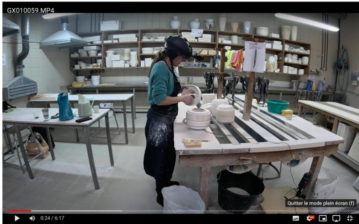
0'41" Using her hand and the scalpel, she continues to remove the excess slip from the middle part of the mould, spinning the whirler.
