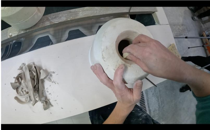
5'16'' She opens the mould by moving the cutter slightly inside the joint, revealing a piece with rounded shapes.
